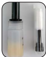
ISE with blank, protective module installed; the sensor module is in a dry, glass vial
